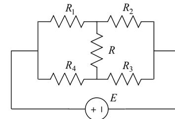
$$\frac{R_1}{R_4} = \frac{R_2}{R_3}$$
