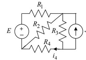
$$\begin{aligned} E &= 54 \text{ V} \\ J &= 10 \text{ A} \\ R_1 &= 6 \Omega & R_2 &= R_3 = 4 \Omega \\ R_4 &= 12 \Omega \end{aligned}$$
