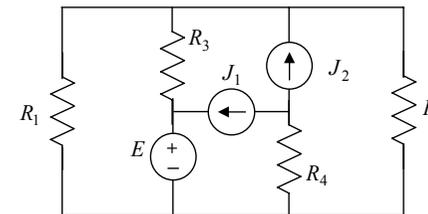
$$J_1 = J_2 = 1 \text{ mA}, \quad E = 2 \text{ mV}$$
