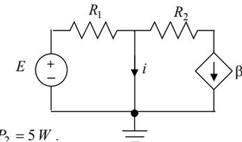
$$E = 6 \text{ V} \\ R_1 = 10 \Omega \quad R_2 = 20 \Omega \\ \beta = 5$$
