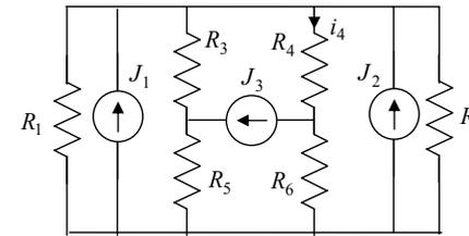
$$\begin{aligned} J_1 = J_2 = 1 \text{ A} \quad J_3 = 3 \text{ A} \\ R_1 = 30 \Omega \quad R_2 = 10 \Omega \\ R_3 = 25 \Omega \quad R_4 = 5 \Omega \\ R_5 = 35 \Omega \quad R_6 = 15 \Omega \end{aligned}$$
