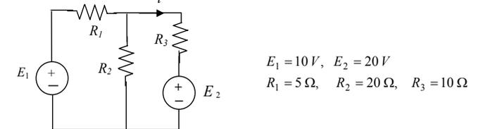
Risultato:  $i = -0.86 \text{ A}, P_{E_1}^{erog} = -2.86 \text{ W}$ .
