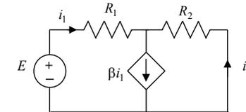
$$\text{Risultato: } I_{cc} = (1 - \beta) \frac{E}{R_1}, \quad R_{eq} = \frac{R_1}{1 - \beta}, \quad i_2 = -I_{cc} \frac{R_{eq}}{R_2 + R_{eq}}.$$
