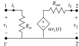
$$G_{11} = \left. \frac{i_1}{v_1} \right|_{v_2=0} = \frac{i_1}{R_{in} i_1} = \frac{1}{R_{in}};$$
