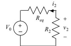
$$R_{eq} = \left. \frac{v_2}{i_2} \right|_{E=0} = \frac{v_2}{\frac{v_2 + 2v_2}{R_1}} = \frac{R_1}{3} = 2 \Omega.$$
