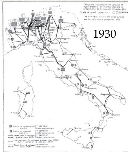
FIG. 4 - Scheme of the Italian electric plants (reproduced from a report issued by the Public Utilities Ministry)
