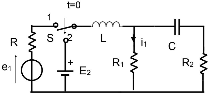
$R_1 = 7 \Omega, R_2 = 3 \Omega, R = 5 \Omega, C = 10/4 \text{ mF}, L = 300 \text{ mH}$
