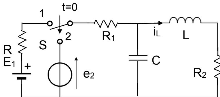
$$R_1 = 8 \, \Omega, R_2 = 2 \, \Omega, R = 5 \, \Omega, C = 10/4 \, \text{mF}, L = 300 \, \text{mH}$$
