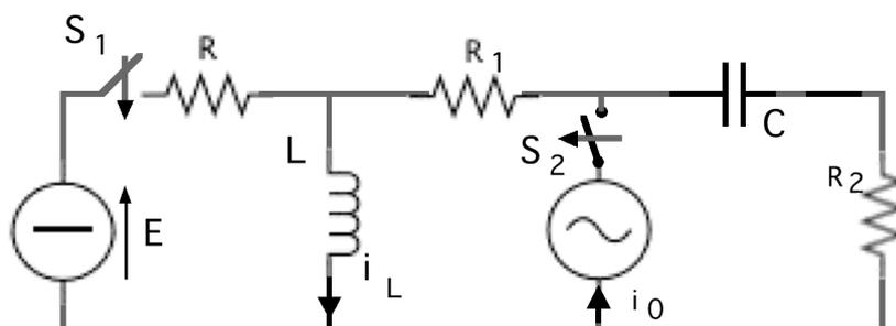
$$R = 100 \, \Omega; R_1 = 20 \, \Omega; R_2 = 30 \, \Omega; C = 1 \, \mu\text{F}; L = 4 \, \text{mH};$$
