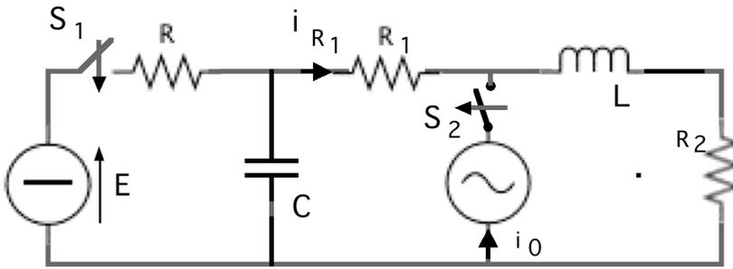
$$R = 100 \, \Omega; R_1 = 30 \, \Omega; R_2 = 20 \, \Omega; C = 1 \, \mu\text{F}; L = 4 \, \text{mH};$$
