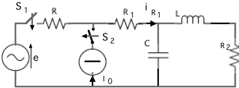
$$R = 10 \Omega; R_1 = 10 \Omega; R_2 = 10 \Omega; C = 1 \mu\text{F}; L = 1 \text{ mH};$$
