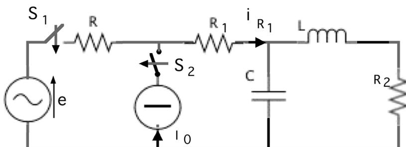
$$R = 20 \Omega; R_1 = 10 \Omega; R_2 = 10 \Omega; C = 1 \mu\text{F}; L = 1 \text{ mH};$$
