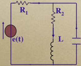
$$Z = R_1 + \frac{-jX_C(R_2 + jX_L)}{R_2 + j(X_L - X_C)}$$
