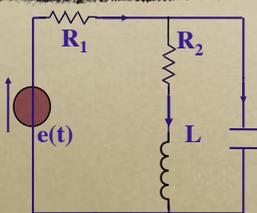
$$\begin{cases} \bar{I}_1 = \bar{I}_2 + \bar{I}_3 \\ \bar{E} = R_1 \bar{I}_1 + (R_2 + jX_L) \bar{I}_2 \\ (R_2 + jX_L) \bar{I}_2 = -jX_C \bar{I}_3 \end{cases}$$
