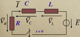
$$\bar{E} = R\bar{I} + j\omega L\bar{I} - j\frac{1}{\omega C}\bar{I}$$
