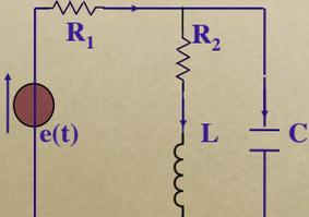
$$\begin{aligned}C &= 1\text{mF}; \\ L &= 50\text{ mH}; \\ R_1 &= 10\ \Omega; \\ R_2 &= 5\ \Omega;\end{aligned}$$
