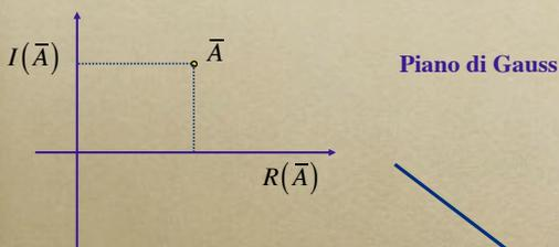
$$\bar{A} = Ae^{j(\omega t + \alpha)} = A \cos(\omega t + \alpha) + jA \sin(\omega t + \alpha)$$
