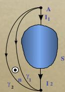
$$\int_{\gamma_1} \vec{E} \cdot d\vec{l} - \int_{\gamma_2} \vec{E} \cdot d\vec{l} = \frac{d}{dt} \iint_S \vec{B} \cdot d\vec{S}$$
