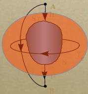
$$\oint_{\gamma_c} \vec{B} \cdot d\vec{l} = \iint_{S_{\gamma_c}} \mu_0 \vec{J} \cdot d\vec{S}$$
