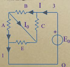
$$\begin{aligned} R_A &= 1 \Omega; \\ R_B &= 1 \Omega; \\ R_C &= 3 \Omega; \\ R_E &= 3 \Omega; \\ R_D &= 3 \Omega; \\ E_0 &= 3V. \end{aligned}$$
