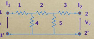
$$G_{11} = \left[ \frac{(R_e + R_2) R_4}{R_2 + R_e + R_4} + R_1 \right]^{-1}$$
