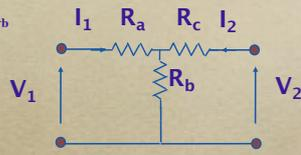
$$\begin{aligned} R_a &= 2 \Omega; \\ R_b &= 2 \Omega; \\ R_c &= 1 \Omega. \end{aligned}$$
