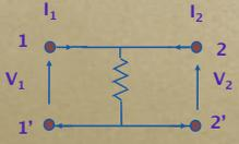
$$G_{12} = \left. \frac{I_1}{V_2} \right|_{V_1=0}$$
