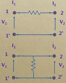
$$R_{12} = \left. \frac{V_1}{I_2} \right|_{I_1=0}$$
