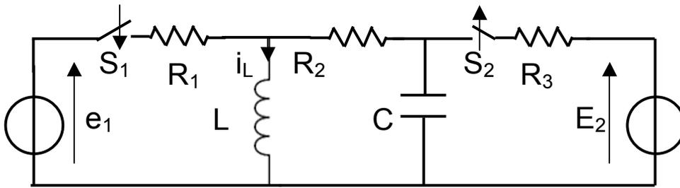
$$R_1 = 6 \, \Omega, R_2 = 3 \, \Omega, R_3 = 7 \, \Omega, C = 10/3 \, \text{mF}, L = 300 \, \text{mH}$$
