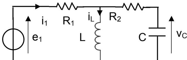
$$Z = R_1 + \frac{jX_L(R_2 - jX_C)}{R_2 + j(X_L - X_C)}$$
