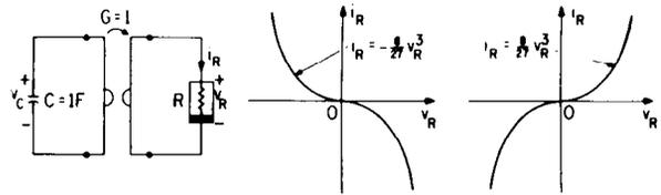
Fig. 25. A gyrator network which does not have a local  $C^1$  state equation at  $q_C = v_L = 0$ .
