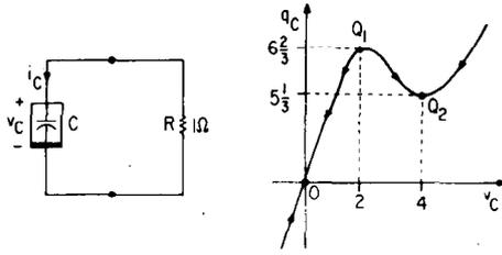
Fig. 3. The  $q_C-v_C$  curve for voltage-controlled capacitor  $C$  of Example 3. Here  $v_C$  is a global coordinate for this curve. The capacitor charge  $q_C$  does not qualify as a global coordinate. Nor does it qualify as a local coordinate at  $Q_1$  or  $Q_2$ .
