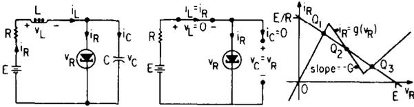
Fig. 10. A dynamic network and its associated resistive network obtained by open-circuiting the capacitor and short-circuiting the inductor.
