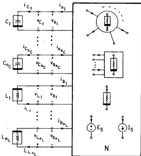
Fig. 20. Any RLC network  $\mathcal{U}$  can be represented by an  $n$ -port resistor  $N$  terminated by  $n_C$  (possibly coupled) capacitors and  $n_L$  (possibly coupled) inductors, where  $n = n_C + n_L$ .
