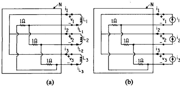
Fig. 22. (a) A 3-inductor autonomous network  $\mathcal{N}$ . (b) The resistive 3-port  $N$  associated with  $\mathcal{N}$  driven by 3 current sources  $i_1, i_2,$  and  $i_3$  corresponding to the 3 inductor currents  $i_{L_1}, i_{L_2},$  and  $i_{L_3}$ .
