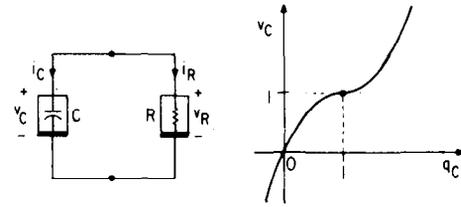
Fig. 1. A 2-element RC network  $\mathcal{N}$  (Example 1).
