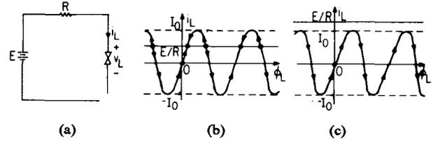
Fig. 11. (a) Josephson junction circuit: The constitutive relation of the nonlinear inductor is given by  $i_L = I_0 \sin k\phi_L$ . (b) Although the resistive circuit has a *unique* operating point, there are infinitely many equilibrium points if  $E < RI_0$ . (c) There are no equilibrium points if  $E > RI_0$ .
