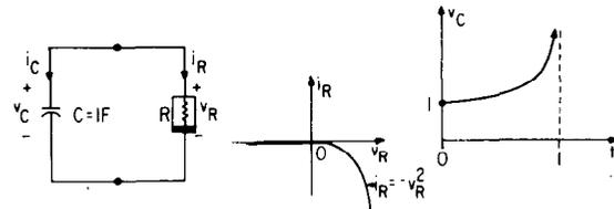
Fig. 8. A *nonphysical* network exhibiting a finite-forward-escape-time solution.
