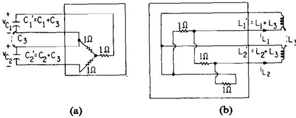
Fig. 24. (a) Equivalent network obtained by open-circuiting capacitor  $C_3$  from Fig. 21(a), thereby eliminating the capacitor loop. (b) Equivalent network obtained by short-circuiting inductor  $L_3$  from Fig. 22(a), thereby eliminating the inductor cut set.
