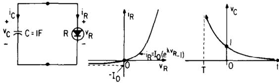
Fig. 9. A network exhibiting a finite-backward-escape-time solution.
