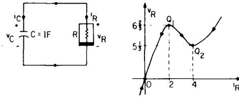
Fig. 4. The  $i_R-v_R$  curve for current-controlled resistor  $R$  of Example 4. Here  $i_R$  is a global coordinate for this curve. The resistor voltage  $v_R$  does not qualify as a global coordinate. Nor does it qualify as a local coordinate at  $Q_1$  or  $Q_2$ .
