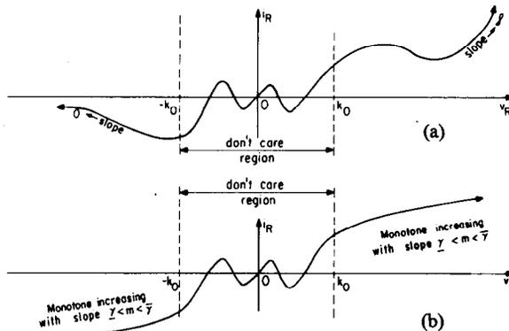
Fig. 27. (a) The  $v_R-i_R$  curve of an eventually passive 2-terminal resistor. (b) The  $v_R-i_R$  curve of an eventually strongly locally passive 2-terminal resistor.
