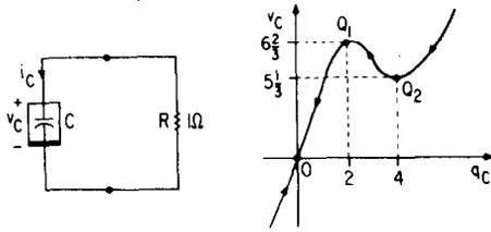
Fig. 2. The  $q_C-v_C$  curve for charge-controlled capacitor  $C$  of Example 2. Here  $q_C$  is a global coordinate for this curve. The capacitor voltage  $v_C$  does not qualify as a global coordinate. Nor does it qualify as a "local" coordinate at  $Q_1$  or  $Q_2$ .
