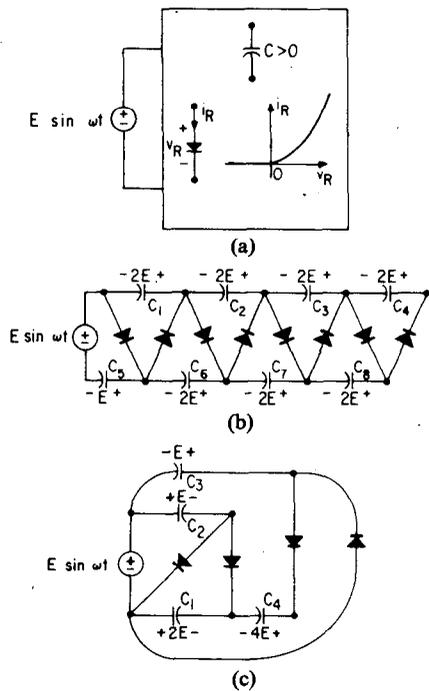
Fig. 34. (a) A diode-capacitor network driven by a sinusoidal voltage source. (b) A ladder-type dc voltage multiplier. (c) A voltage-quadrupler having the smallest "output" resistance.
