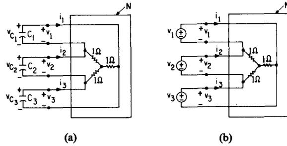
Fig. 21. (a) A 3-capacitor autonomous RC network  $\mathcal{N}$ . (b) The resistive 3-port  $N$  associated with  $\mathcal{N}$  driven by 3 voltage sources  $v_1, v_2$ , and  $v_3$  corresponding to the 3 capacitor voltages  $v_{C_1}, v_{C_2}$ , and  $v_{C_3}$ .
