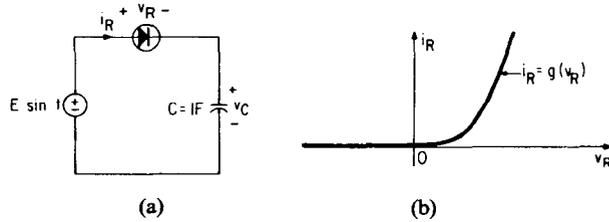
Fig. 17. A network (driven by a periodic source) having infinitely many distinct periodic solutions depending only on the initial voltage  $v_C(0) < E$ .
