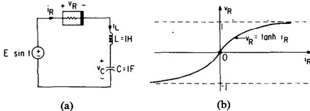
Fig. 16. A network made of strictly passive and strictly locally passive elements driven by a sinusoidal voltage source can give an unbounded zero-state solution.
