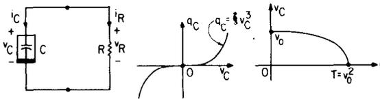
Fig. 6. A network having no solution for  $t > v_0^2$ . However, the solution exists and is bounded for  $0 < t < v_0^2$ .
