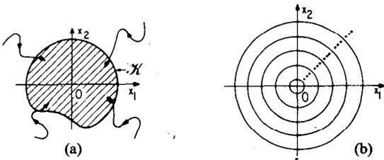
Fig. 30. (a) All trajectories must eventually enter and remain inside the closed and bounded set  $\mathcal{X}$ . (b) A continuum of periodic orbits, one for each initial condition.
