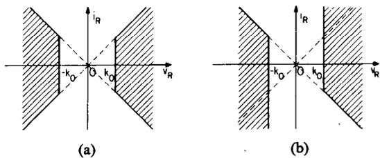
Fig. 26. (a) If the  $v_R-i_R$  curve lies within the shaded region for all  $|v_R| > k_0$ , the network in Figs. 8 and 9 have no finite-forward and backward escape-time solutions. (b) If the  $v_R-i_R$  curve lies within the expanded shaded region for all  $|v_R| > k_0$ , the network in Figs. 8 and 9 have no finite-forward-escape-time solutions.
