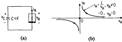
Fig. 15. A passive network having a bounded capacitor charge and voltage solution but an unbounded resistor current solution.
