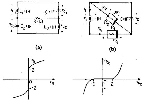
Fig. 28. (a) An oscillatory network which satisfies all hypotheses except condition 1 of *Theorem 12*. (b) An oscillatory network which satisfies all hypotheses except condition 2 of *Theorem 12*, when  $R_1$  and  $R_2$  are described as in (c) and (d).
