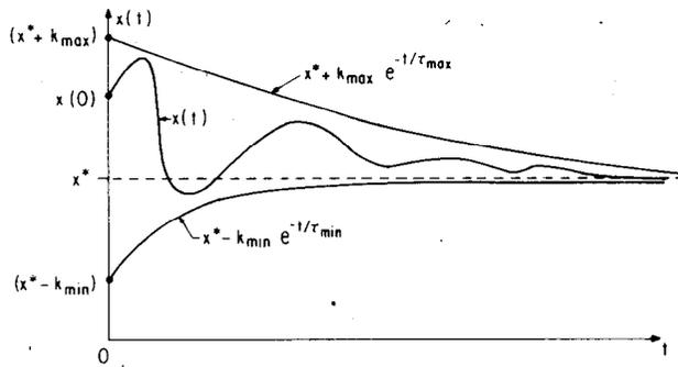
Fig. 33. A geometrical interpretation of *Theorem 21* for a first order network: The solution  $x(t)$  is bounded by 2 exponentials having time constants  $\tau_{\min}$  and  $\tau_{\max}$ , respectively.
