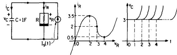
Fig. 7. A network with infinitely many solutions all of which having the same initial voltage  $v_C(0) = 3$ .
