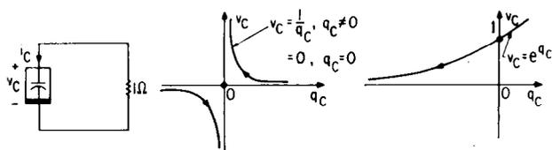
Fig. 14. A network having an *unbounded* capacitor voltage solution when the  $q_C-v_C$  curve is as shown in Fig. 14(b), and *unbounded* capacitor charge solution when the  $q_C-v_C$  curve is as shown in Fig. 14(c).
