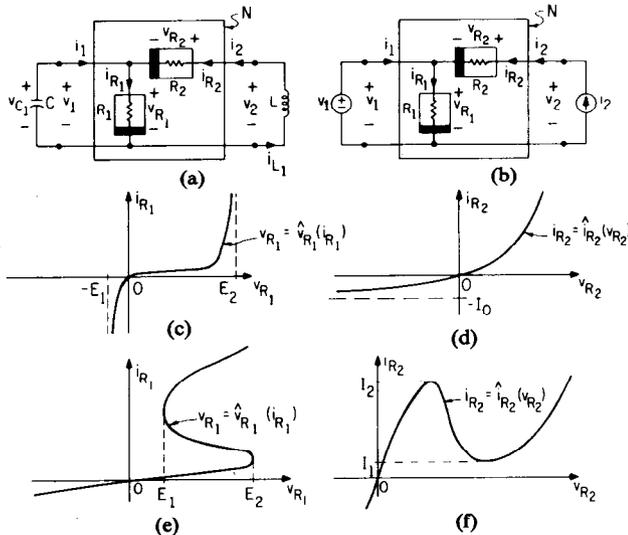
Fig. 23. (a) An autonomous  $RC$  network  $\mathcal{N}$ . (b) The resistive 2-port  $N$  associated with  $\mathcal{N}$  driven by a voltage source  $v_1$  (corresponding to capacitor  $C$ ) and a current source  $i_2$  (corresponding to inductor  $L$ ). (c) A typical "Zener diode"  $v_{R_1}-i_{R_1}$  curve. (d) A typical "p-n junction diode"  $v_{R_2}-i_{R_2}$  curve. (e) A typical "neon bulb"  $v_{R_1}-i_{R_1}$  curve. (f) A typical "tunnel diode"  $v_{R_2}-i_{R_2}$  curve.
