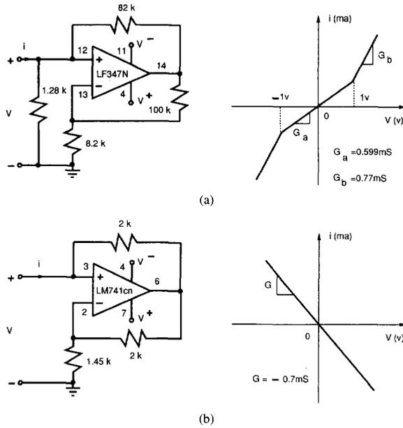
Fig. 9. (a) Implementation of nonlinear resistor  $N_r$ ; (b) implementation of negative linear resistor  $R$ .
