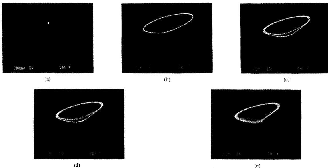
Fig. 4. Phase portraits in  $v_{C_1} - v_{C_2}$  plane of a typical period-doubling sequence.  $C_1 = 5.75nF$ ,  $C_2 = 21.32nF$ ,  $L = 12mH$ ,  $R_0 = 30.86\Omega$ ,  $G_a = -0.879mS$ ,  $G_b = -0.4124mS$  and  $E = 1V$ : (a) Equilibrium point,  $R > 1.558k\Omega$ ; (b) period-1 limit cycle,  $R = 1.558k\Omega$ ; (c) period-2 limit cycle,  $R = 1.516k\Omega$ ; (d) period-4 limit cycle,  $R = 1.508k\Omega$ ; (e) spiral Chua's attractor,  $R = 1.503k\Omega$ .
