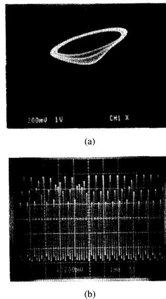
Fig. 6. (a) Intermittency of type I. Parameters are the same as in Fig. 4 except  $R$ . Phase portraits in  $v_{C_1} - v_{C_2}$  plane of intermittency near a period-3 window,  $R = 1.502k\Omega$ ; (b) time waveform of  $v_{C_1}$  of intermittency near a period-3 window,  $R = 1.502k\Omega$ .
