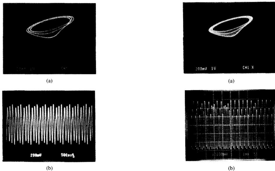
Fig. 5. Intermittency near a period-3 limit cycle. Parameters are the same as in Fig. 4 except  $R$ : (a) Phase portraits in  $v_{C_1} - v_{C_2}$  plane of a period-3 limit cycle,  $R = 1.501k\Omega$ ; (b) time waveform of  $v_{C_1}$  of a period-3 limit cycle,  $R = 1.501k\Omega$ .
