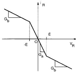
Fig. 3. Typical  $v-i$  characteristic of Chua's diode.
