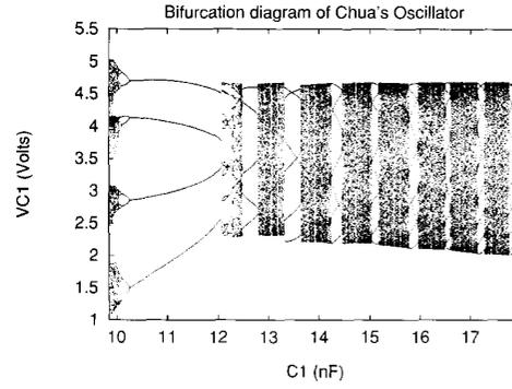
Fig. 13. Bifurcation diagram of torus breakdown sequence.
