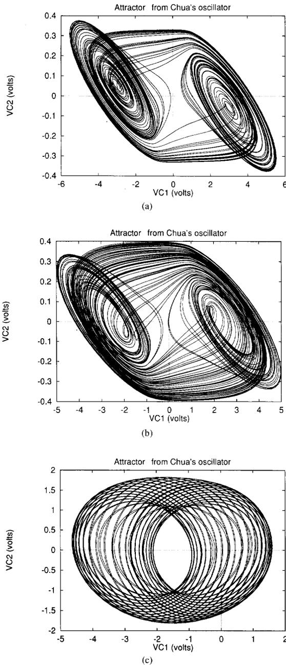
Fig. 11. Computer generated phase portrait in  $v_{C_1} - v_{C_2}$  plane of attractors in Fig. 10.  $G_a = 0.599mS, G_b = 0.77mS, G = \frac{1}{R} = -0.7mS, E = 1V$ : (a)  $C_1 = 0.0135\mu F, C_2 = 1.9319\mu F, L = 19mH, R_0 = 26.7\Omega$ ; (b)  $C_1 = 0.019\mu F, C_2 = 0.285\mu F, L = 2.056mH, R_0 = 12.5\Omega$ ; (c)  $C_1 = 0.0297\mu F, C_2 = 0.3606\mu F, L = 7.682mH, R_0 = 13.4\Omega$ .
