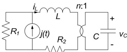
$$R_1 = 10 \Omega; R_2 = 10 \Omega;$$
