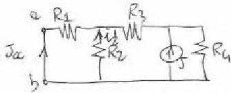
$$R_1 J_{ca} = i_2' R_2, \quad i_2' = \frac{R_1 J_{ca}}{R_2} = \frac{3}{2} \cdot (-2)$$
