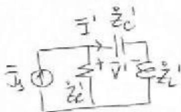
$\bar{I}' = \bar{I}_1 \frac{\bar{Z}'_C}{\bar{Z}'_R + \bar{Z}'_{eq}} = 1 \frac{1}{1 - 3,75i}$
