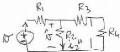
$$R_{eq} = R_2 \parallel (R_3 + R_4) = \frac{2 \cdot 2}{4} = 1$$
