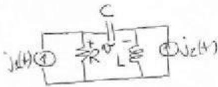
$i_1(t) = I_{m1} \cos(\omega_1 t), i_2(t) = I_{m2} \sin(\omega_2 t)$
