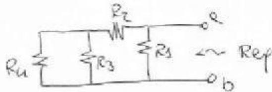
$$R_{eq}^{(1)} = R_4 \parallel R_3 = 1,$$
