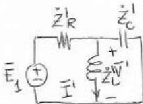
$$\bar{V}' = \bar{E}_1 \frac{\bar{Z}_{eq}'^{(1)}}{\bar{Z}_R' + \bar{Z}_{eq}'^{(1)}} = 1 \frac{\frac{i}{3,75}}{1 + \frac{i}{3,75}} = \frac{i}{i + 3,75}$$
