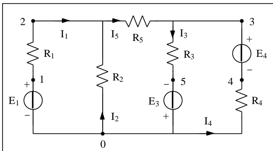
Dati:  $E_1 = 10 \text{ V}$ ,  $E_3 = 70 \text{ V}$ ,  $E_4 = -20 \text{ V}$ ,  $R_1 = 10 \text{ } \Omega$ ,  $R_2 = 5 \text{ } \Omega$ ,  $R_3 = 2 \text{ } \Omega$ ,  $R_4 = 4 \text{ } \Omega$ ,  $R_5 = 1 \text{ } \Omega$ .
