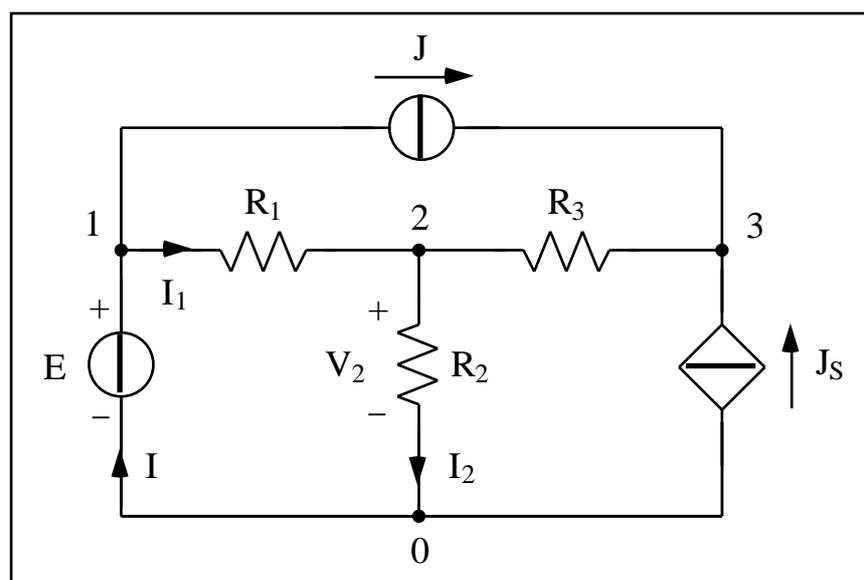
Dati:  $E = 20 \text{ V}$ ,  $J = 30 \text{ A}$ ,  $R_1 = 1$ ,  $R_2 = 2$ ,  $R_3 = 3$ ,  $J_s = V_2$ ,  $\beta = 0.25 \text{ S}$ .
