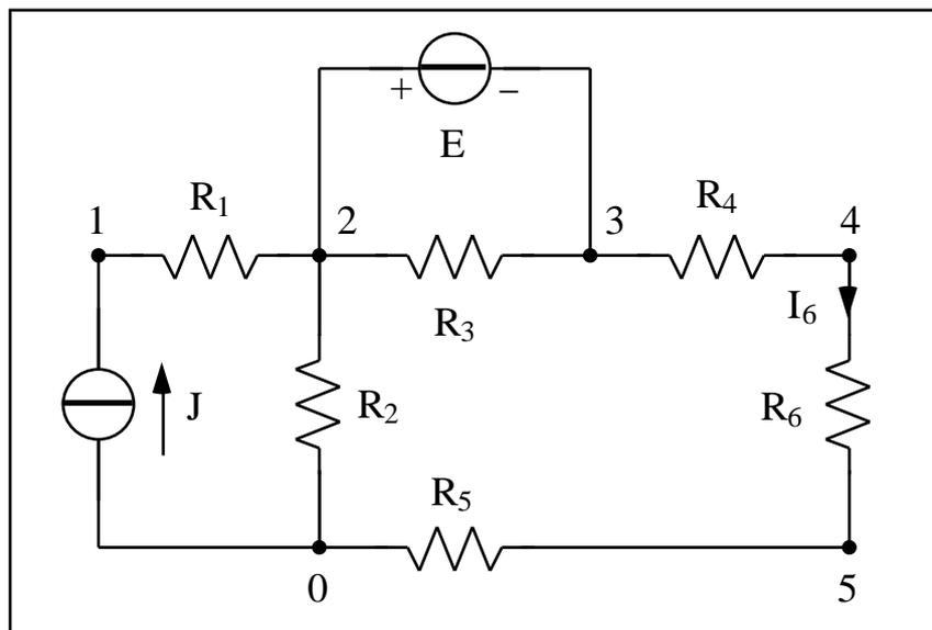
Dati:  $J = 5 \text{ A}$ ,  $E = 340 \text{ V}$ ,  $R_1 = 8 \text{ } \Omega$ ,  $R_2 = 20 \text{ } \Omega$ ,  $R_3 = 80 \text{ } \Omega$ ,  $R_4 = 5 \text{ } \Omega$ ,  $R_5 = 10 \text{ } \Omega$ ,  $R_6 = 45 \text{ } \Omega$ .
