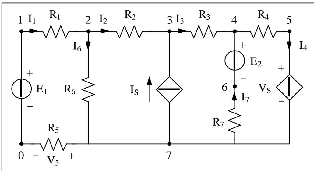
Dati:  $E_1 = 16 \text{ V}$ ,  $E_2 = 12 \text{ V}$ ,  $V_S = V_5$ ,  $\beta = 3$ ,  $I_S = I_4$ ,  $\alpha = 2$ ,  $R_1 = 3 \ \Omega$ ,  $R_2 = 2 \ \Omega$ ,  $R_3 = 6 \ \Omega$ ,  $R_4 = 7 \ \Omega$ ,  $R_5 = 5 \ \Omega$ ,  $R_6 = 1 \ \Omega$ ,  $R_7 = 4 \ \Omega$ .
