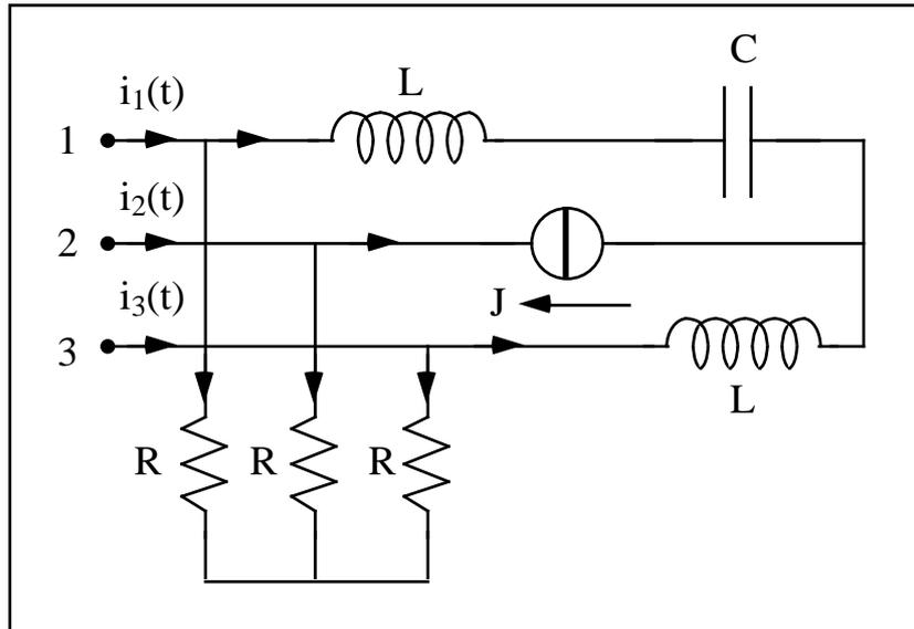
Dati:  $v_{12}(t) = V_0 \cos(\omega t)$ ,  $V_0 = 200\sqrt{6}$  V,  $\omega = 500$  rad/s,  $J = 10$  A,  $R = 5 \Omega$ ,  $L = 1$  mH,  $C = 4$  mF.
