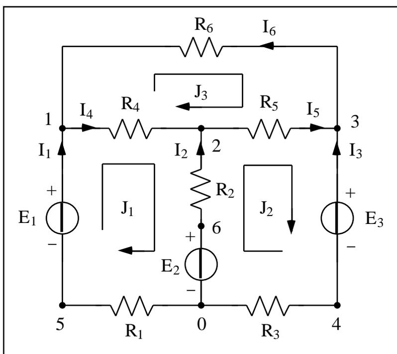
Dati:  $E_1 = 460 \text{ V}$ ,  $E_2 = 230 \text{ V}$ ,  $E_3 = 115 \text{ V}$ ,  $R_1 = 8 \text{ } \Omega$ ,  $R_2 = 4 \text{ } \Omega$ ,  $R_3 = 10 \text{ } \Omega$ ,  $R_4 = 2 \text{ } \Omega$ ,  $R_5 = 6 \text{ } \Omega$ ,  $R_6 = 12 \text{ } \Omega$ .
