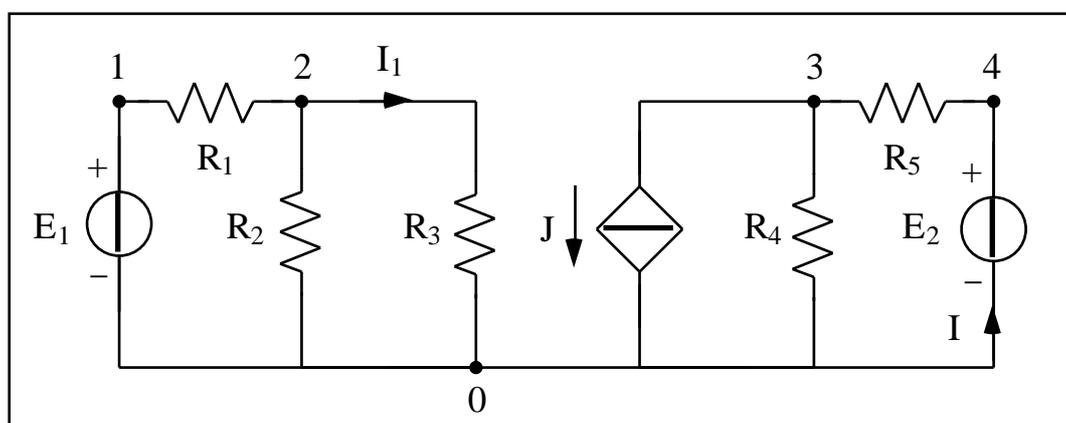
Dati:  $E_1 = 20 \text{ V}$ ,  $E_2 = 7 \text{ V}$ ,  $J = 5 \text{ A}$ ,  $I_1 = 2/3 \text{ A}$ ,  $R_1 = 2 \text{ } \Omega$ ,  $R_2 = 4 \text{ } \Omega$ ,  $R_3 = 12 \text{ } \Omega$ ,  $R_4 = 3 \text{ } \Omega$ ,  $R_5 = 6 \text{ } \Omega$ .
