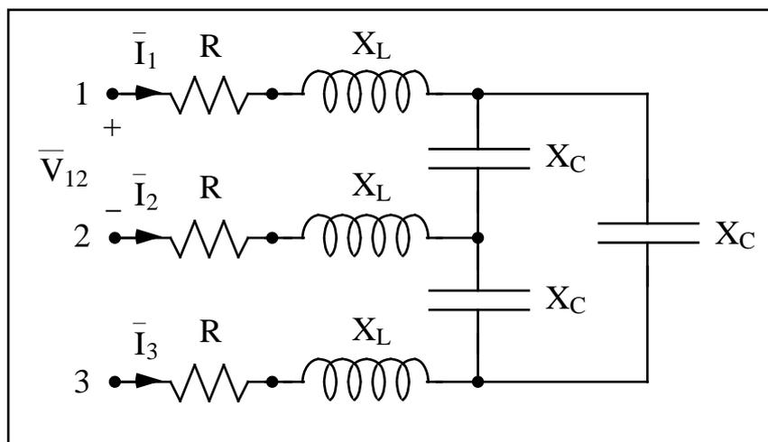
Dati:  $\bar{V}_{12} = 200\sqrt{3}$  V,  $R = 5$   $\Omega$ ,  $X_L = 2$   $\Omega$ ,  $X_C = 6$   $\Omega$ .
