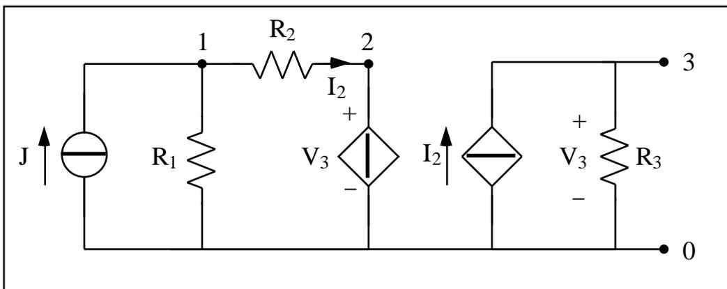
Dati:  $J = 135 \text{ nA}$ ,  $R_1 = 100$  ,  $R_2 = 980$  ,  $R_3 = 40 \text{ k}$  ,  $\beta = 5 \cdot 10^{-5}$  ,  $\alpha = 40$ .
