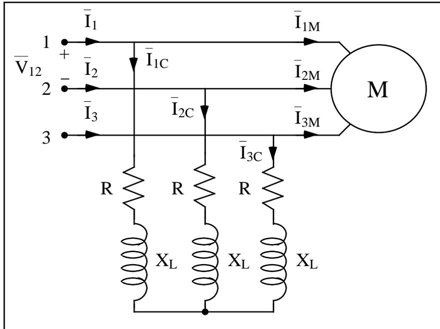
Dati:  $\bar{V}_{12} = 220 \sqrt{3} \text{ V}$ ,  $P_M = 1.5 \text{ kW}$ ,  $Q_M = 1.5 \text{ kVAr}$ ,  $R = X_L = 10 \text{ } \Omega$ .
