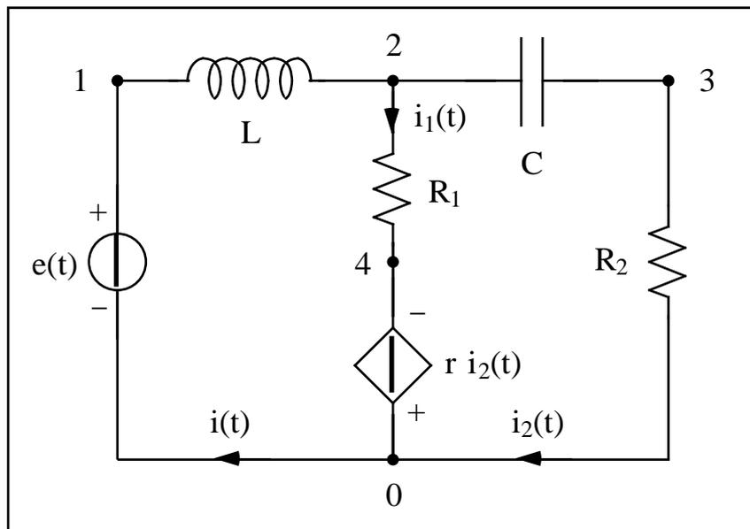
Dati:  $e(t) = E \cos(\omega t)$ ,  $E = 130 \text{ V}$ ,  $\omega = 10 \text{ krad/s}$ ,  $r = 30$ ,  $R_1 = 40 \Omega$ ,  $R_2 = 100 \Omega$ ,  $L = 5 \text{ mH}$ ,  $C = 2 \mu\text{F}$ .
