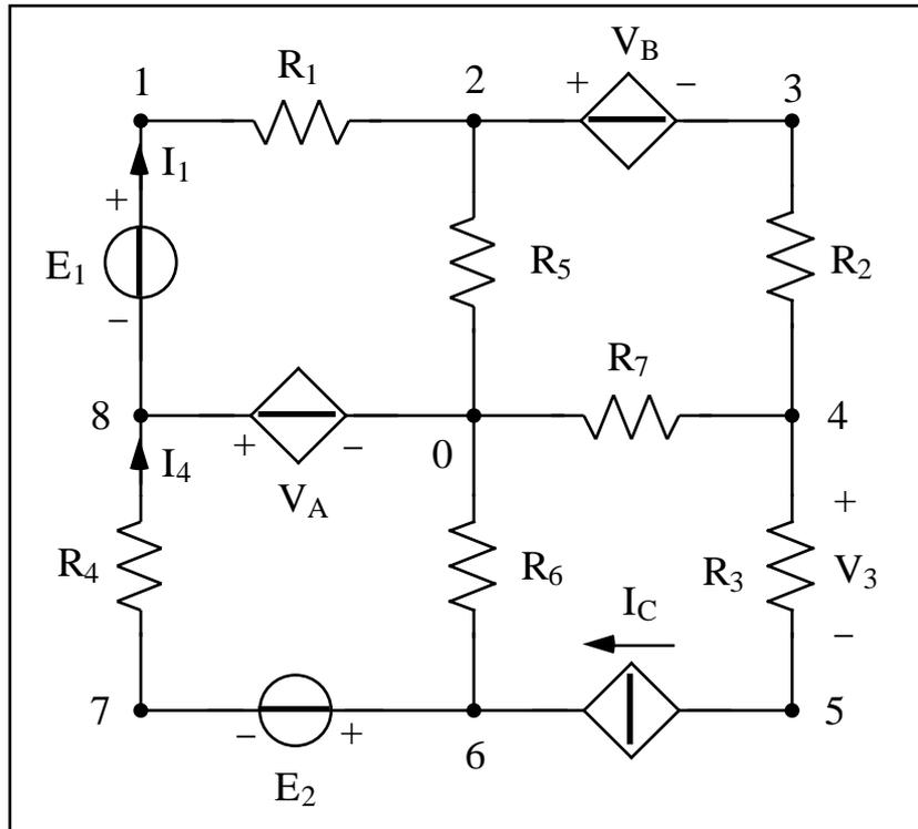
Dati:  $E_1 = 10 \text{ V}$ ,  $E_2 = 6 \text{ V}$ ,  $V_A = I_4$ ,  $V_B = V_3$ ,  $I_C = I_1$ ,  $R_1 = 7 \text{ } \Omega$ ,  $R_2 = 4 \text{ } \Omega$ ,  $R_3 = 6 \text{ } \Omega$ ,  $R_4 = 1 \text{ } \Omega$ ,  $R_5 = 5 \text{ } \Omega$ ,  $R_6 = 2 \text{ } \Omega$ ,  $R_7 = 3 \text{ } \Omega$ .
