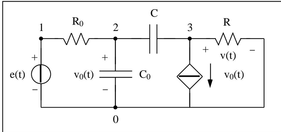
Dati:  $e(t) = E \sin(\omega t)$ ,  $E = 10 \text{ V}$ ,  $\omega = 1 \text{ krad/s}$ ,  $R_0 = 100 \Omega$ ,  $C_0 = 10 \mu\text{F}$ ,
