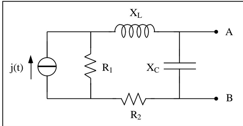
Dati:  $\bar{J} = 16 \text{ A}$ ,  $R_1 = 25 \text{ } \Omega$ ,  $R_2 = 15 \text{ } \Omega$ ,  $X_L = 30 \text{ } \Omega$ ,  $X_C = 50 \text{ } \Omega$ .
