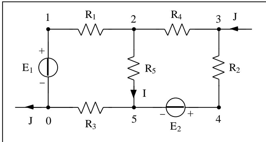
Dati:  $E_1 = 60 \text{ V}$ ,  $E_2 = 130 \text{ V}$ ,  $J = 12 \text{ A}$ ,  $R_1 = R_5 = 2 \ \Omega$ ,  $R_2 = R_3 = 5 \ \Omega$ ,  $R_4 = 4 \ \Omega$ .
