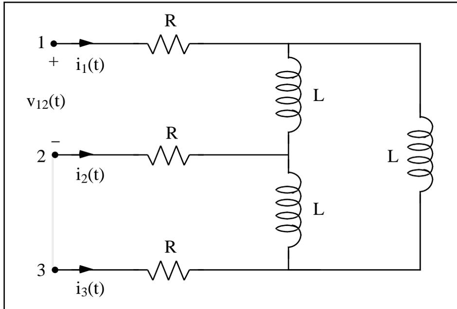
Dati:  $v_{12}(t) = V_0 \cos(\omega t + \pi/4)$ ,  $V_0 = 12\sqrt{6}$  V,  $\omega = 300$  rad/s,  $R = 3$   $\Omega$ ,  $L = 30$  mH.
