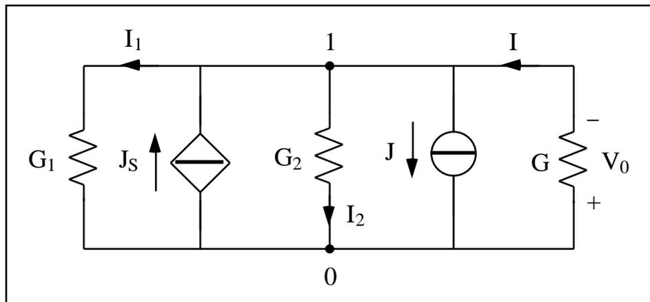
Dati:  $J = 20 \text{ A}$ ,  $J_s = I_1 = 2$ ,  $G_1 = 1/4 \text{ S}$ ,  $G_2 = 1/3 \text{ S}$ ,  $V_0 = 24 \text{ V}$ .
