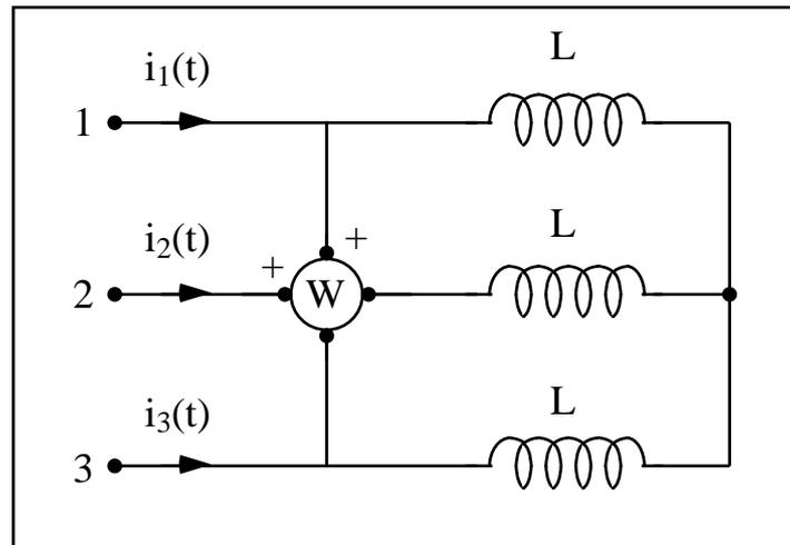
Dati:  $i_2(t) = I_0 \sqrt{2} \sin(\omega t)$ ,  $I_0 = 20 \text{ A}$ ,  $\omega = 100 \text{ rad/s}$ ,  $L = 1 \text{ mH}$ .
