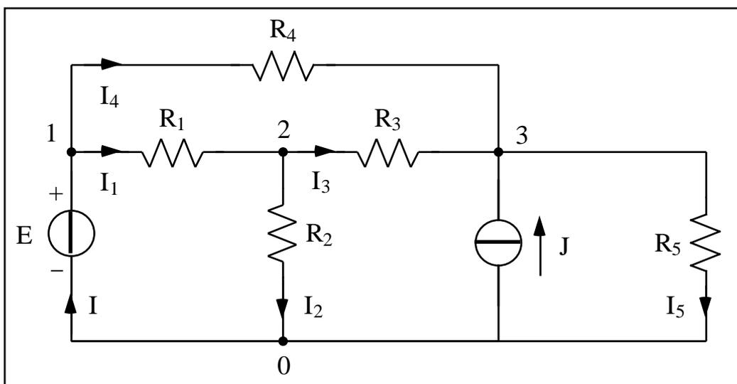
Dati:  $E = 50 \text{ V}$ ,  $J = 1 \text{ A}$ ,  $R_1 = 80 \text{ } \Omega$ ,  $R_2 = 50 \text{ } \Omega$ ,  $R_3 = 40 \text{ } \Omega$ ,  $R_4 = 800 \text{ } \Omega$ ,  $R_5 = 200 \text{ } \Omega$ .
