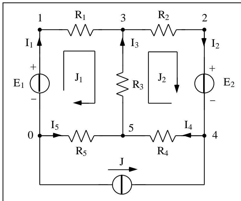
Dati:  $E_1 = 600 \text{ V}$ ,  $E_2 = 400 \text{ V}$ ,  $J = 12 \text{ A}$ ,  $R_1 = 10 \ \Omega$ ,  $R_2 = 8 \ \Omega$ ,  $R_3 = 40 \ \Omega$ ,  $R_4 = 14 \ \Omega$ ,  $R_5 = 2 \ \Omega$ .
