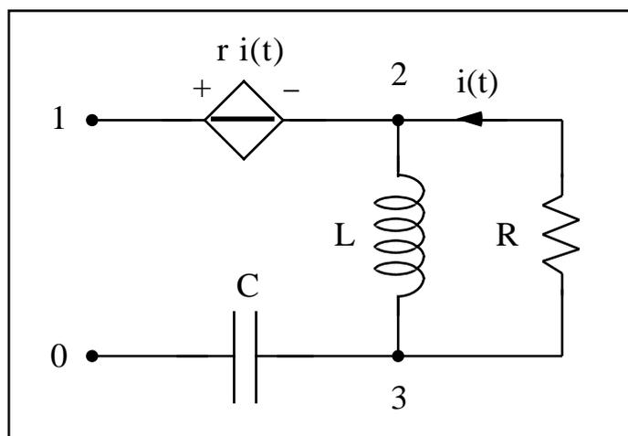
Dati:  $R = 30 \ \Omega$ ,  $L = 0.6 \text{ mH}$ ,  $C = 0.4 \ \mu\text{F}$ ,  $r = 5$ ,  $\omega = 100 \text{ krad/s}$ .
