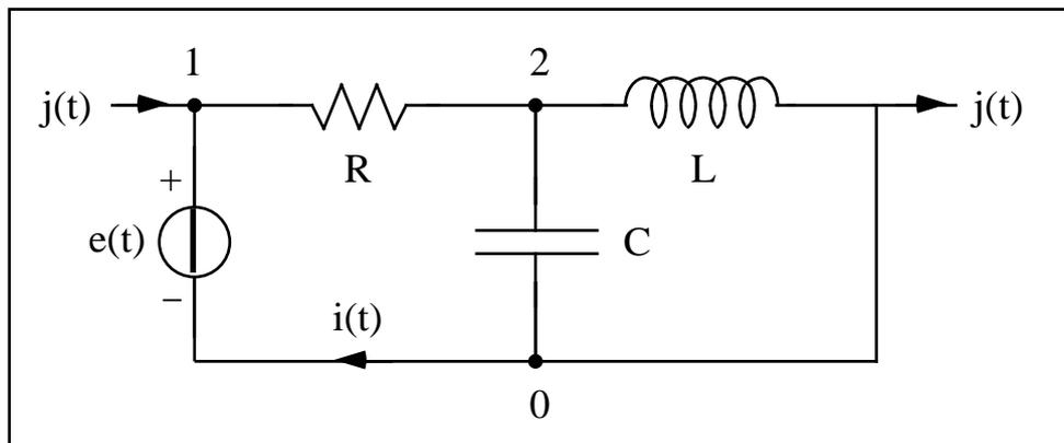
Dati:  $j(t) = I \cos(\omega_1 t)$ ,  $e(t) = E \cos(\omega_2 t)$ ,  $I = 4 \text{ A}$ ,  $E = 3\sqrt{2} \text{ V}$ ,  $\omega_1 = 1 \text{ krad/s}$ ,  $\omega_2 = 3\omega_1$ ,  $R = 0.75 \Omega$ ,  $L = 2 \text{ mH}$ ,  $C = 0.5 \text{ mF}$ .
