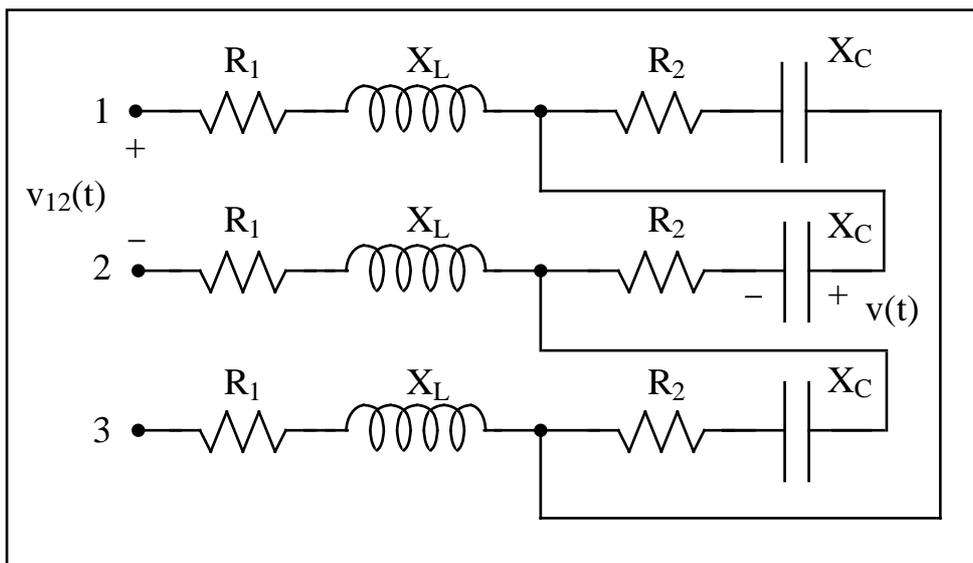
Dati:  $v(t) = V_0 \text{ sen}( \omega t - \pi/3)$ ,  $V_0 = 330 \sqrt{2} \text{ V}$ ,  $R_1 = X_L = 5 \text{ } \Omega$ ,  $R_2 = X_C = 15 \text{ } \Omega$ .
