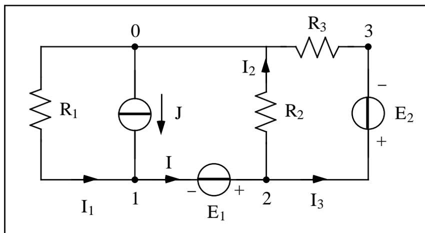
Dati:  $E_1 = 12 \text{ V}$ ,  $E_2 = 6 \text{ V}$ ,  $J = 5 \text{ A}$ ,  $R_1 = 15 \text{ } \Omega$ ,  $R_2 = 3 \text{ } \Omega$ ,  $R_3 = 6 \text{ } \Omega$ .
