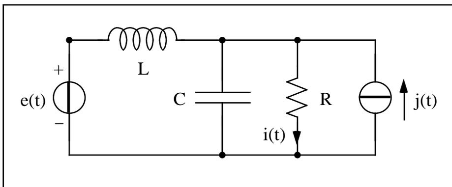
Dati:  $T = 0.02 \text{ s}$ ,  $\omega = 2\pi/T$ ,  $e(t) = E \cos(\omega t)$ ,  $i(t) = I \cos(\omega t)$ ,  $I = 2 \text{ A}$ ,  $R = 20 \Omega$ ,  $L = 8 \text{ mH}$ ,  $C = 0.4 \text{ nF}$ .
