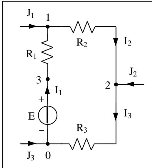
Dati:  $E = 20 \text{ V}$ ,  $J_1 = 10 \text{ A}$ ,  $J_2 = -20 \text{ A}$ ,  $R_1 = 10 \ \Omega$ ,  $R_2 = 2 \ \Omega$ ,  $R_3 = 3 \ \Omega$ .
