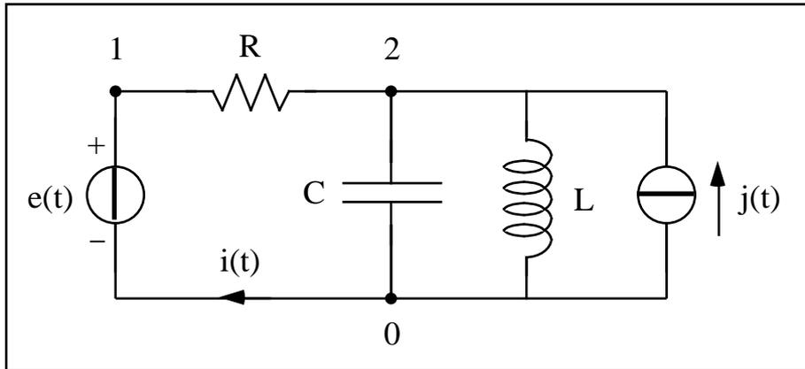
Dati:  $e(t) = E = 5 \text{ V}$ ,  $j(t) = I \cos(\omega t)$ ,  $I = 2 \text{ A}$ ,  $\omega = 1 \text{ krad/s}$ ,  $R = 1 \text{ }\Omega$ ,  $L = 1 \text{ mH}$ ,  $C = 1 \text{ mF}$ .
