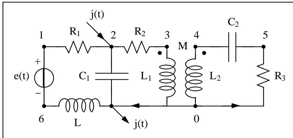
Dati:  $e(t) = 100\sqrt{2} \sin(\omega t)$ ,  $j(t) = -20 \cos(\omega t + \pi/4)$ ,  $\omega = 1 \text{ krad/s}$ ,
