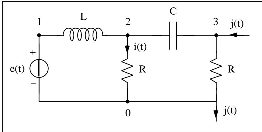
Dati:  $e(t) = E \sin(\omega t)$ ,  $E = 10 \text{ V}$ ,  $j(t) = I \cos(\omega t)$ ,  $I = 2 \text{ A}$ ,  $\omega = 10 \text{ krad/s}$ ,
