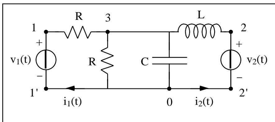
Dati:  $v_1(t) = 10 \cos(1000t)$ ,  $v_2(t) = 20 \sin(1000t)$ ,  $R = 1 \ \Omega$ ,  $L = 1 \text{ mH}$ ,  $C = 1 \text{ mF}$ .
