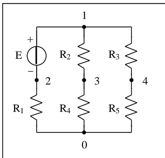
Dati:  $E = 200 \text{ V}$  ,  $R_1 = 10 \text{ R}$  ,  $R_2 = 14 \text{ R}$  ,  $R_3 = 2 \text{ R}$  ,  $R_4 = 6 \text{ R}$  ,  $R_5 = 18 \text{ R}$  .
