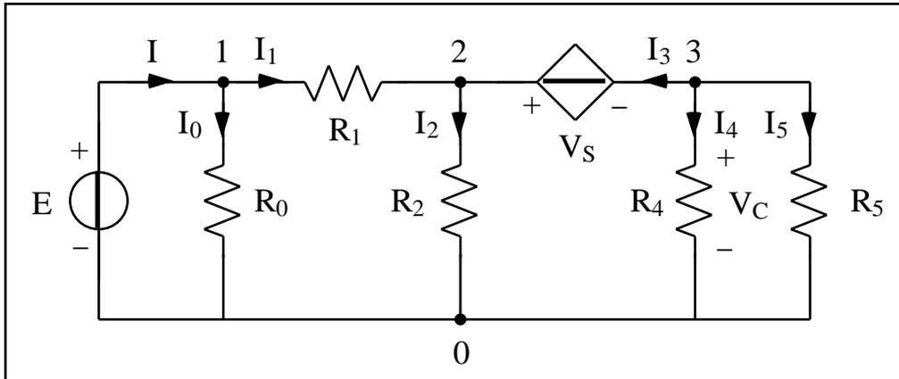
Dati:  $E = 100 \text{ V}$ ,  $V_S = V_C$ ,  $\beta = 4$ ,  $R_0 = 80 \text{ } \Omega$ ,  $R_1 = 10 \text{ } \Omega$ ,  $R_2 = 60 \text{ } \Omega$ ,  $R_4 = 20 \text{ } \Omega$ ,  $R_5 = 30 \text{ } \Omega$ .
