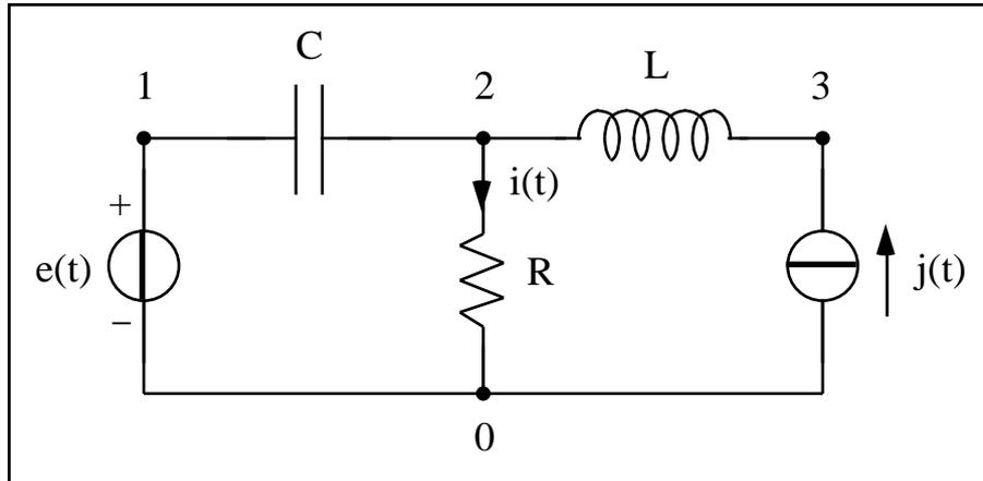
Dati:  $e(t) = E \sin(\omega t)$ ,  $j(t) = -I \cos(\omega t)$ ,  $E = 10 \text{ V}$ ,  $I = 2 \text{ mA}$ ,  $\omega = 200 \text{ rad/s}$ ,
