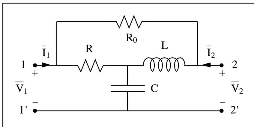
Dati :  $\omega = 1 \text{ krad/s}$ ,  $R = 2 \text{ } \Omega$  ,  $R_0 = 2 \text{ } \Omega$  ,  $L = 2 \text{ mH}$ ,  $C = 1 \text{ mF}$ .
