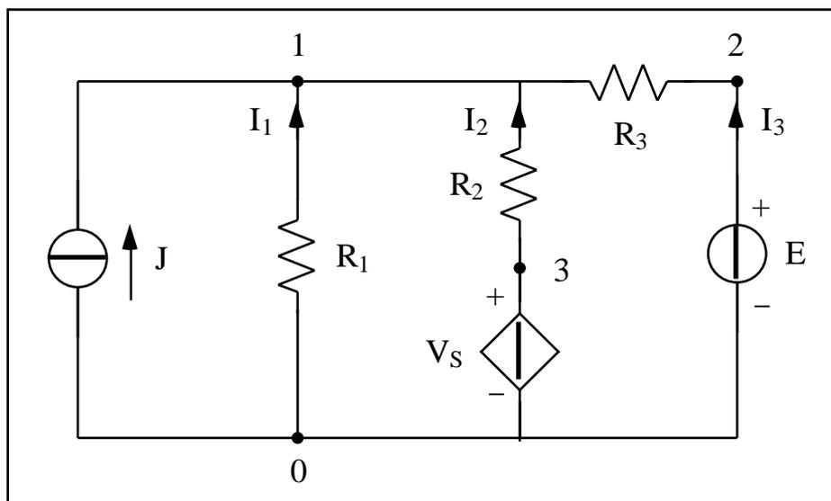
Dati:  $E = 45 \text{ V}$ ,  $J = 0.45 \text{ A}$   $V_S = r I_3$ ,  $r = 6.25$  ,  $R_1 = 100$  ,  $R_2 = 5$  ,  $R_3 = 25$  .
