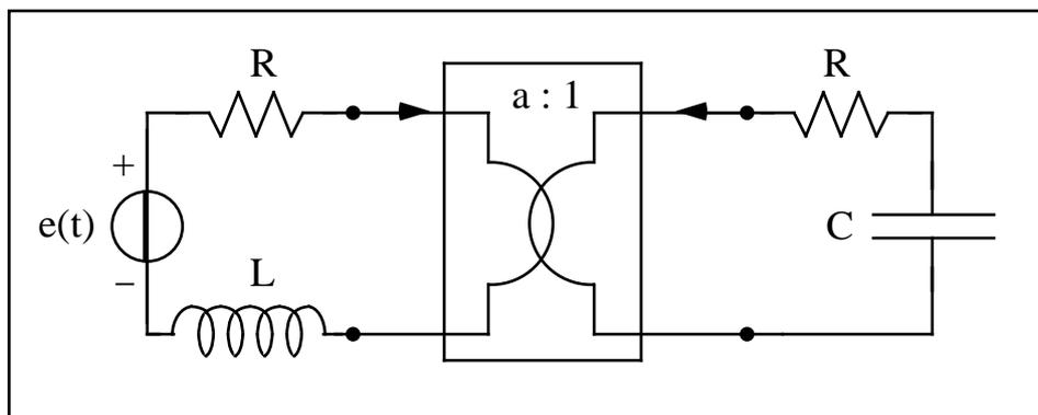
Dati:  $e(t) = E \cos(\omega t)$ ,  $E = 16.4 \text{ V}$ ,  $\omega = 200 \text{ rad/s}$ ,  $R = 10 \text{ } \Omega$ ,  $L = 64 \text{ mH}$ ,  $C = 0.25 \text{ mF}$ ,  $a = 0.8$ .
