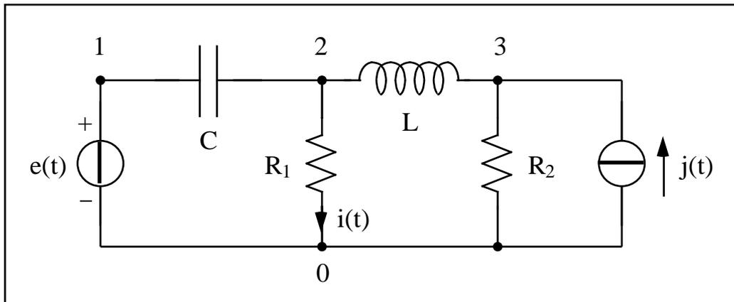
Dati:  $e(t) = E \sin(\omega_1 t)$ ,  $j(t) = I \cos(\omega_2 t)$ ,  $E = 6 \text{ V}$ ,  $I = 4\sqrt{17} \text{ A}$ ,  $T = 8 \text{ ms}$ ,
