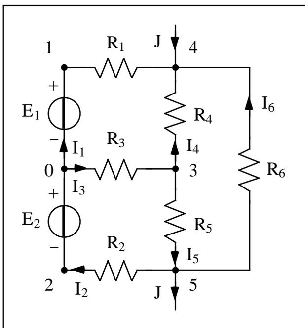
Dati:  $E_1 = 28 \text{ V}$ ,  $E_2 = 40 \text{ V}$ ,  $J = -10 \text{ A}$ ,  $R_1 = 4 \ \Omega$ ,  $R_2 = R_3 = 2 \ \Omega$ ,  $R_4 = 3 \ \Omega$ ,  $R_5 = 8 \ \Omega$ ,  $R_6 = 1 \ \Omega$ .
