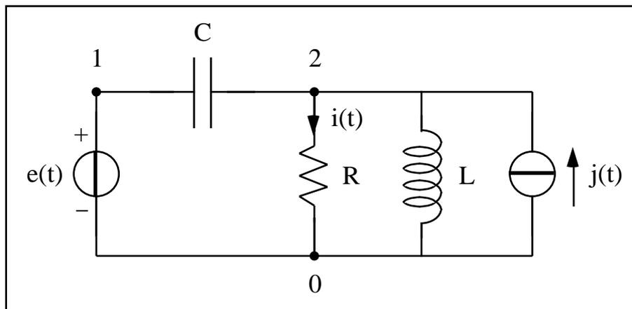
Dati:  $e(t) = E \sin(\omega t)$ ,  $E = 1 \text{ V}$ ,  $j(t) = -I \cos(\omega t)$ ,  $I = 1 \text{ A}$ ,  $\omega = 1 \text{ krad/s}$ ,  $R = 2 \text{ } \Omega$ ,  $L = 1 \text{ mH}$ ,  $C = 1/2 \text{ mF}$ .
