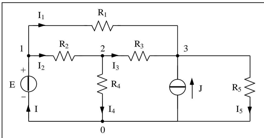
Dati:  $E = 50 \text{ V}$ ,  $J = 0.75 \text{ A}$ ,  $R_1 = 800 \text{ } \Omega$ ,  $R_2 = 80 \text{ } \Omega$ ,  $R_3 = 40 \text{ } \Omega$ ,  $R_4 = 50 \text{ } \Omega$ ,  $R_5 = 200 \text{ } \Omega$ .
