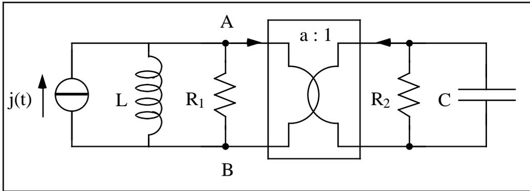
Dati:  $j(t) = I \cos(\omega t)$ ,  $I = 1 \text{ A}$ ,  $\omega = 1 \text{ Mrad/s}$ ,  $R_1 = 200 \text{ } \Omega$ ,  $R_2 = 2 \text{ } \Omega$ ,  $L = 200 \text{ } \mu\text{H}$ ,  $C = 1.5 \text{ } \mu\text{F}$ ,  $a = 10$ .
