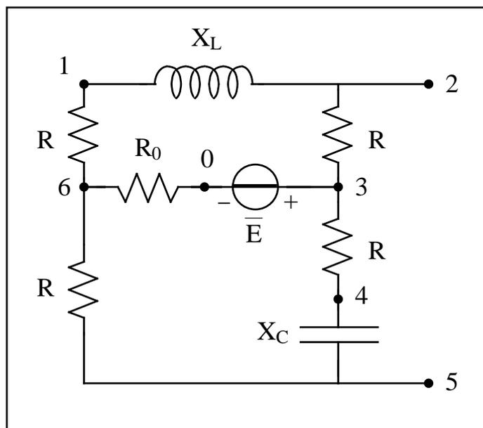
Dati:  $\bar{E} = 60 \text{ V}$ ,  $R_0 = 1 \text{ } \Omega$ ,  $R = 4 \text{ } \Omega$ ,  $X_L = 4 \text{ } \Omega$ ,  $X_C = 4 \text{ } \Omega$ .
