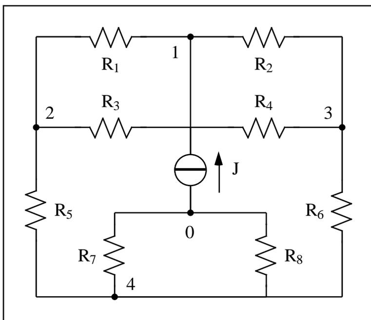
Dati:  $J = 2 \text{ A}$ ,  $R_1 = 150 \text{ } \Omega$ ,  $R_2 = 100 \text{ } \Omega$ ,  $R_3 = 150 \text{ } \Omega$ ,  $R_4 = 100 \text{ } \Omega$ ,  $R_5 = 25 \text{ } \Omega$ ,  $R_6 = 50 \text{ } \Omega$ ,  $R_7 = R_8 = 20 \text{ } \Omega$ .
