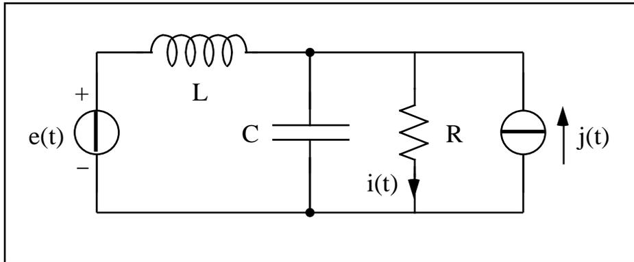
Dati:  $T = 0.02$ ,  $\omega = 2\pi/T$ ,  $e(t) = E \cos(\omega t)$ ,  $j(t) = I \cos(\omega t)$ ,  $I = 2$ ,  $R = 20$ ,  $L = 8 \text{ mH}$ ,  $C = 0.4 \text{ nF}$ .
