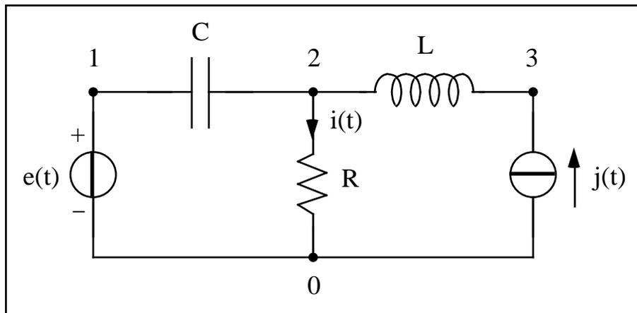
Dati:  $e(t) = E \operatorname{sen}(\omega t)$ ,  $E = 10$ ,  $j(t) = -I \cos(\omega t)$ ,  $I = 2 \text{ mA}$ ,  $\omega = 2000$ ,  $R = 5 \text{ k}\Omega$ ,  $L = 5 \text{ mH}$ ,  $C = 1 \mu\text{F}$ .
