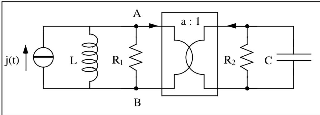
Dati:  $j(t) = I \cos(\omega t)$ ,  $I = 1$ ,  $\omega = 1 \text{ Mrad/s}$ ,  $R_1 = 200$ ,  $R_2 = 2$ ,  $L = 200 \mu\text{H}$ ,  $C = 1.5 \mu\text{F}$ ,  $a = 10$ .
