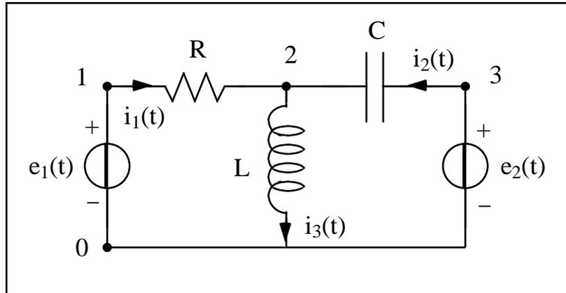
Dati:  $e_1(t) = E_1 \cos(\omega t)$ ,  $e_2(t) = E_2 \sin(\omega t)$ ,  $E_1 = E_2 = 10$ ,  $\omega = 1 \text{ krad/s}$ ,  $R = 5$ ,  $L = 5 \text{ mH}$ ,  $C = 0.2 \text{ mF}$ .
