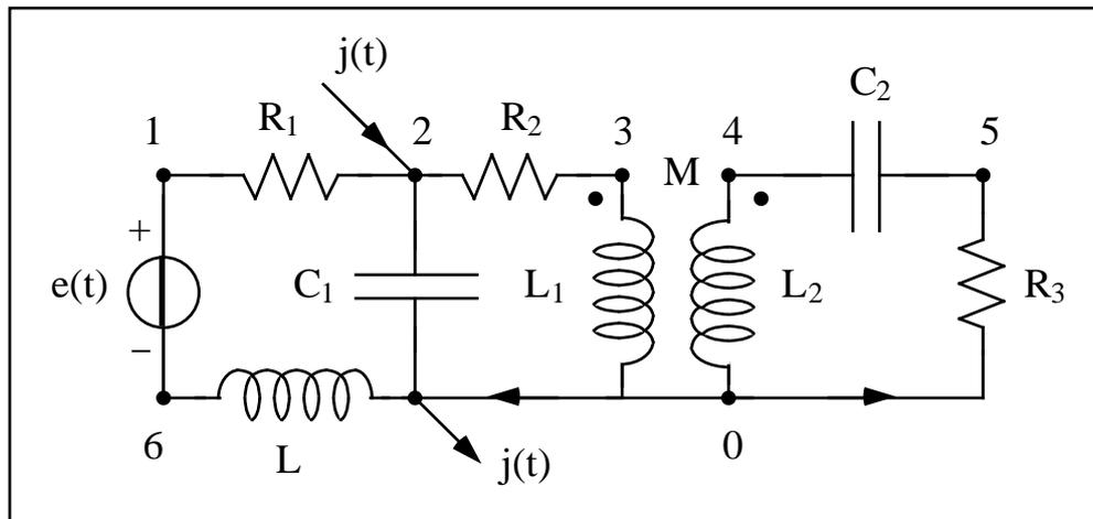
Dati:  $e(t) = E \sin(\omega t)$ ,  $E = 100\sqrt{2}$ ,  $j(t) = -J \cos(\omega t + \phi/4)$ ,  $J = 20$ ,  $\omega = 1$  krad/s,  $R_1 = R_2 = 10$ ,  $R_3 = 2.5$ ,  $L = 5$  mH,  $C_1 = 0.1$  mF,  $C_2 = 0.4$  mF,  $L_1 = 10$  mH,  $L_2 = 2.5$  mH,  $|M| = 5$  mH.
