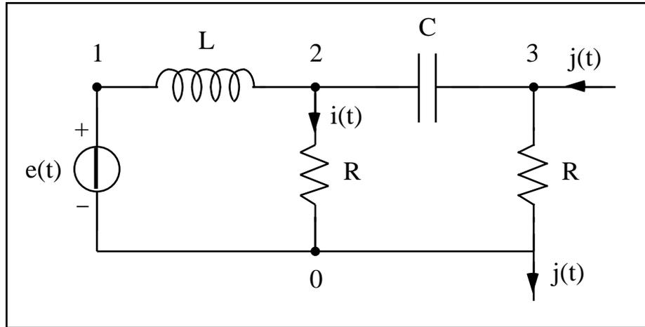
Dati:  $e(t) = E \sin(\omega t)$ ,  $E = 10$ ,  $j(t) = I \cos(\omega t)$ ,  $I = 2$ ,  $\omega = 10 \text{ krad/s}$ ,  $R = 10$ ,  $L = 1 \text{ mH}$ ,  $C = 10 \mu\text{F}$ .
