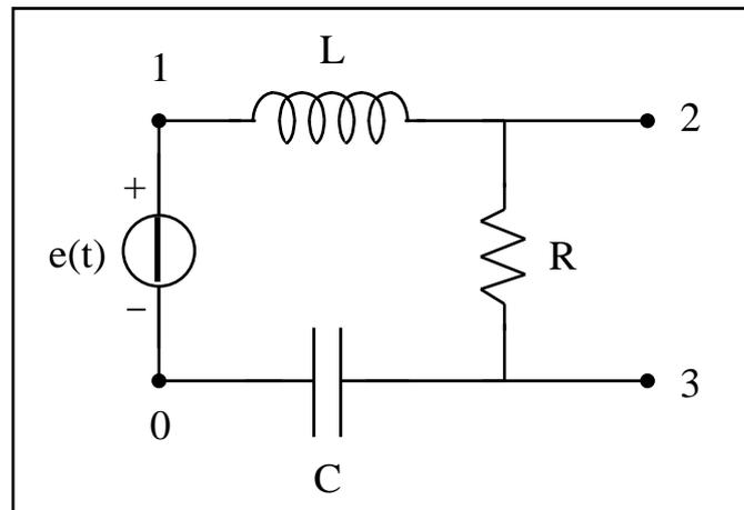
Dati:  $e(t) = E \cos(\omega t)$ ,  $E = 100$ ,  $\omega = 20 \text{ krad/s}$ ,  $R = 10$ ,  $L = 1 \text{ mH}$ ,  $C = 5 \mu\text{F}$ .
