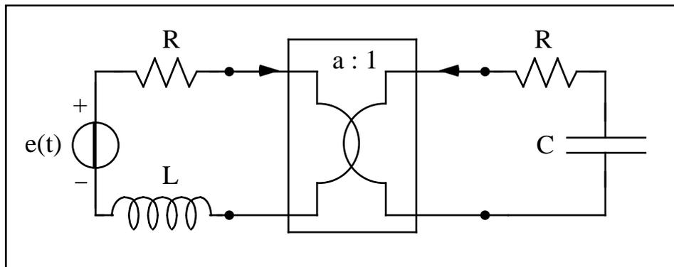
Dati:  $e(t) = E \cos(\omega t)$ ,  $E = 16.4 \text{ V}$ ,  $\omega = 200 \text{ rad/s}$ ,  $R = 10$ ,  $L = 64 \text{ mH}$ ,  $C = 0.25 \text{ mF}$ ,  $a = 0.8$ .
