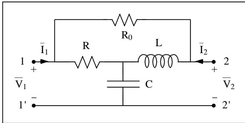
Dati :  $\omega = 1 \text{ krad/s}$ ,  $R = 2$ ,  $R_0 = 2$ ,  $L = 2 \text{ mH}$ ,  $C = 1 \text{ mF}$ .
