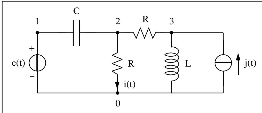
Dati:  $e(t) = E \sin(100t)$ ,  $E = 1$ ,  $j(t) = I \cos(100t)$ ,  $I = 1$ ,  $R = 1$ ,  $R = 1$ ,  $C = 10 \text{ mF}$ ,  $L = 10 \text{ mH}$ .
