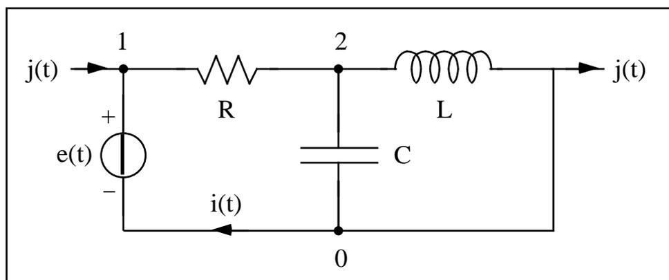
Dati:  $j(t) = I \cos(\omega_1 t)$ ,  $e(t) = E \cos(\omega_2 t)$ ,  $I = 4$ ,  $E = 3\sqrt{2}$ ,  $\omega_1 = 1 \text{ krad/s}$ ,  $\omega_2 = 3\omega_1$ ,  $R = 0.75$ ,  $L = 2 \text{ mH}$ ,  $C = 0.5 \text{ mF}$ .
