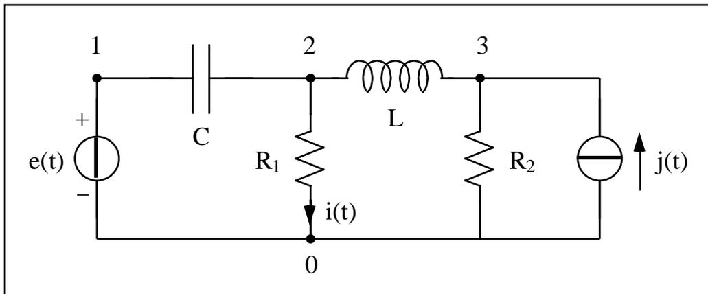
Dati:  $e(t) = E \sin(\omega_1 t)$ ,  $j(t) = I \cos(\omega_2 t)$ ,  $E = 6$ ,  $I = 4\sqrt{17}$ ,  $T = 8$  ms,  $\omega_1 = 2\pi/T$ ,  $\omega_2 = 2\pi/T$ ,  $R_1 = R_2 = 2$ ,  $L = 8$  mH,  $C = 4$  mF.
