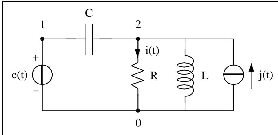
Dati:  $e(t) = E \sin(\omega t)$ ,  $E = 1$ ,  $j(t) = -I \cos(\omega t)$ ,  $I = 1$ ,  $\omega = 1 \text{ krad/s}$ ,  $R = 2$ ,  $L = 1 \text{ mH}$ ,  $C = 1/2 \text{ mF}$ .
