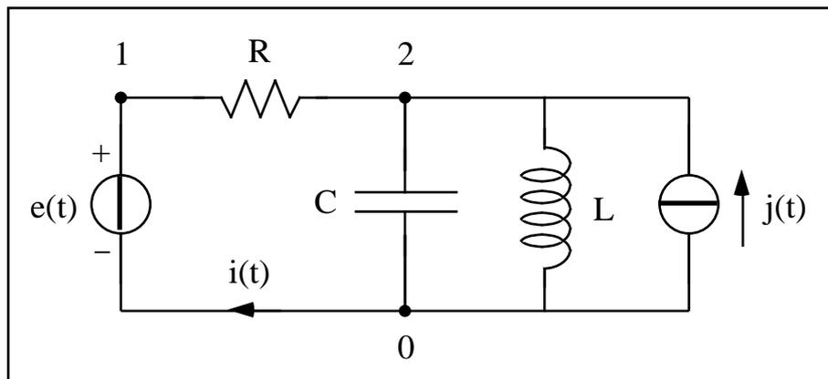
Dati:  $e(t) = E = 5$ ,  $j(t) = I \cos(\omega t)$ ,  $I = 2$ ,  $\omega = 1 \text{ krad/s}$ ,  $R = 1$ ,  $L = 1 \text{ mH}$ ,  $C = 1 \text{ mF}$ .
