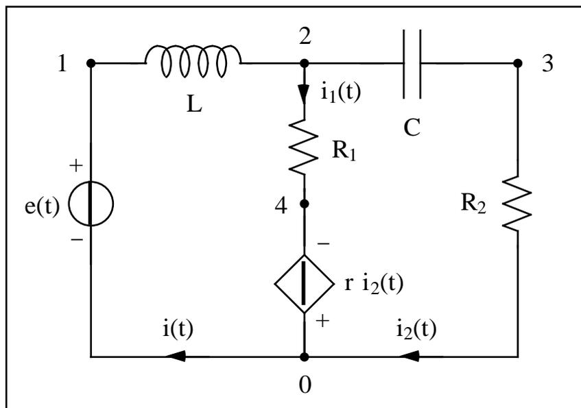
Dati:  $e(t) = E \cos(\omega t)$ ,  $E = 130$ ,  $\omega = 10 \text{ krad/s}$ ,  $r = 30$ ,  $R_1 = 40$ ,  $R_2 = 100$ ,  $L = 5 \text{ mH}$ ,  $C = 2 \text{ }\mu\text{F}$ .
