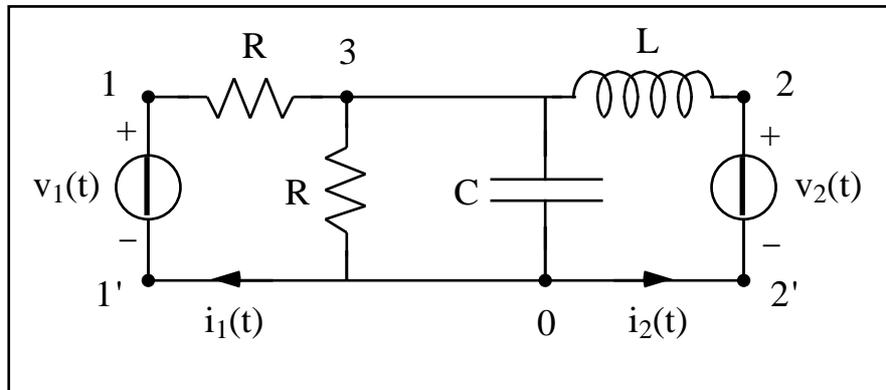
Dati:  $v_1(t) = 10 \cos(1000t)$ ,  $v_2(t) = 20 \sin(1000t)$ ,  $R = 1$ ,  $L = 1 \text{ mH}$ ,  $C = 1 \text{ mF}$ .
