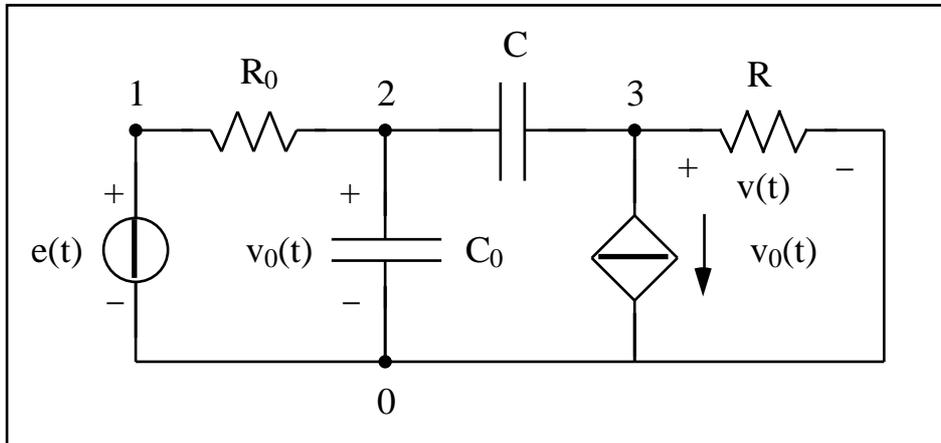
Dati:  $e(t) = E \sin(\omega t)$ ,  $E = 10$ ,  $\omega = 1 \text{ krad/s}$ ,  $R_0 = 100$ ,  $C_0 = 10 \mu\text{F}$ ,  $C = 8 \mu\text{F}$ ,  $R = 1 \text{ k}$ ,  $\beta = 10 \text{ mS}$ .
